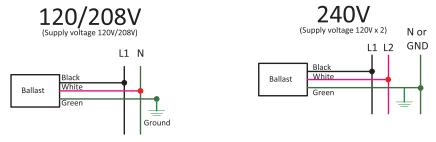
Each ballast **MUST** be wired to the main's neutral line back to the circuit. **DO NOT** "daisy-chain" a neutral line with any other ballast.
